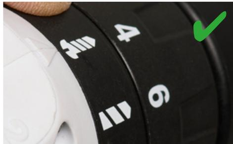
Incorrect setting as driver is set to drill position
