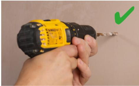
Correct fixing penetration through the board
