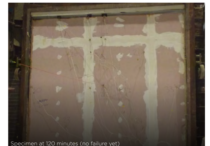
Specimen at 120 minutes (no failure yet)
