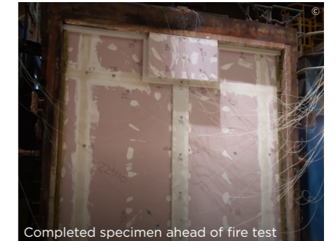
Completed specimen ahead of fire test
