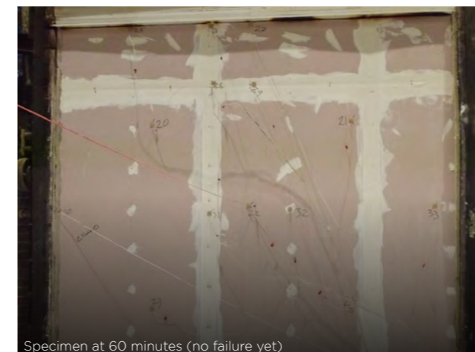
Specimen at 60 minutes (no failure yet)
