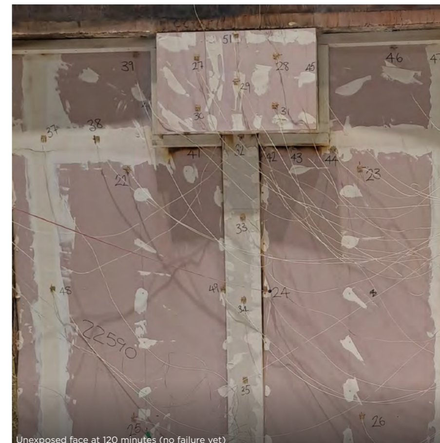
Unexposed face at 120 minutes (no failure yet)
