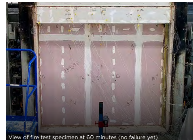
View of fire test specimen at 60 minutes (no failure yet)
