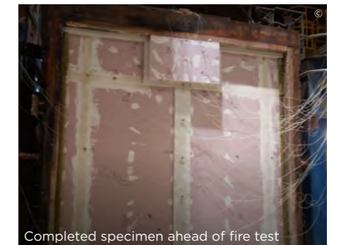
Completed specimen ahead of fire test
