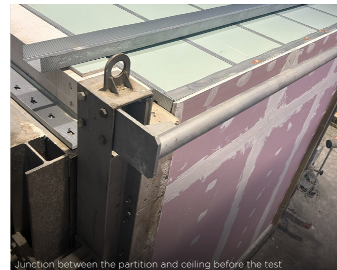
Junction between the partition and ceiling before the test
