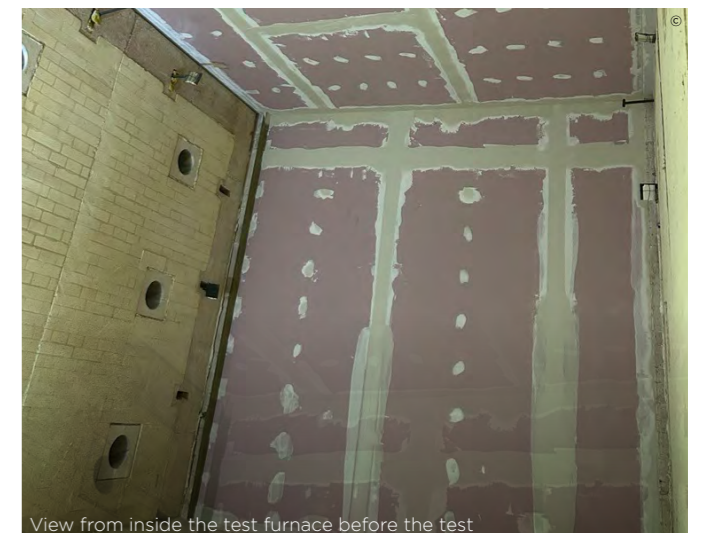
View from inside the test furnace before the test
