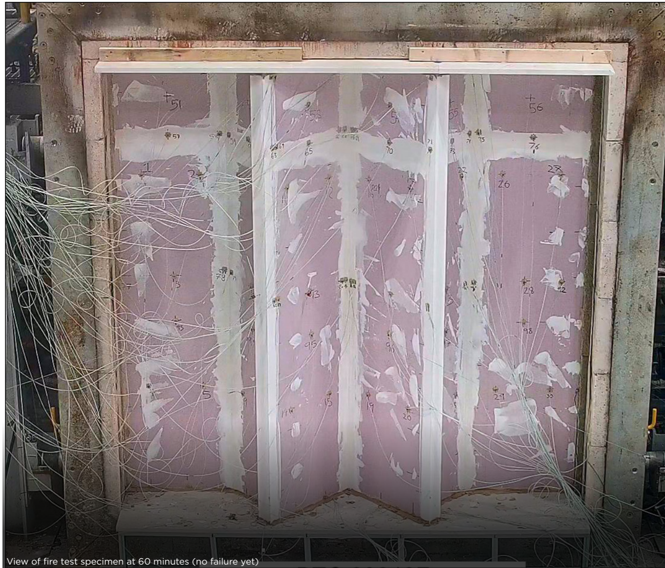
View of fire test specimen at 60 minutes (no failure yet)
