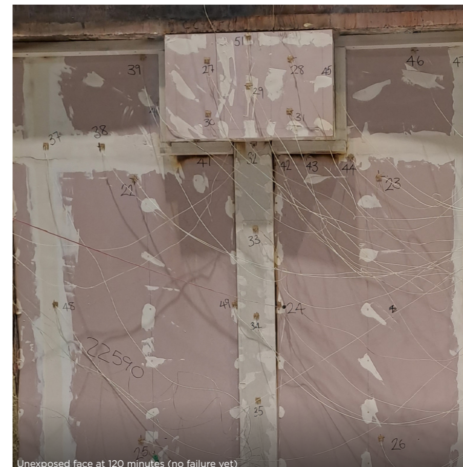
Unexposed face at 120 minutes (no failure yet)
