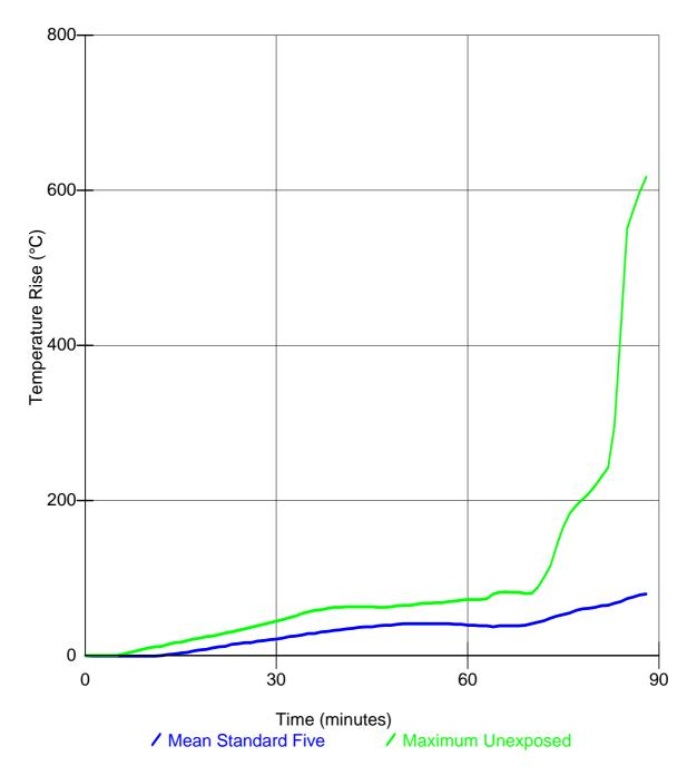
Figure 7 - Unexposed face temperature graph
