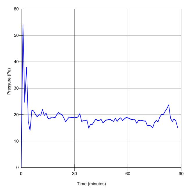
**Figure 6 -** Furnace pressure graph The furnace pressure was set to control at 18  $\pm$  2 Pa positive with respect to atmosphere, at the top of the specimen.
