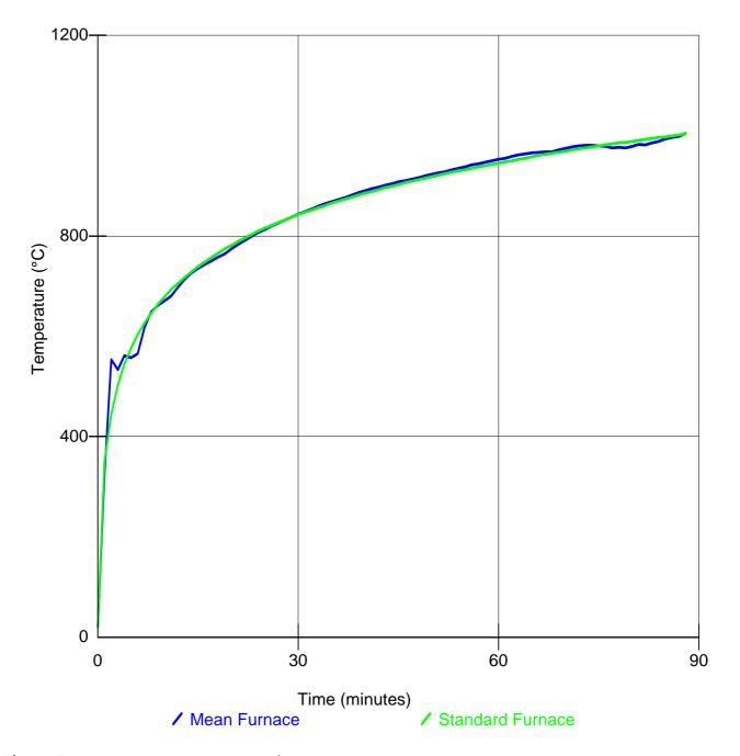
Figure 5 - Furnace temperature graph
