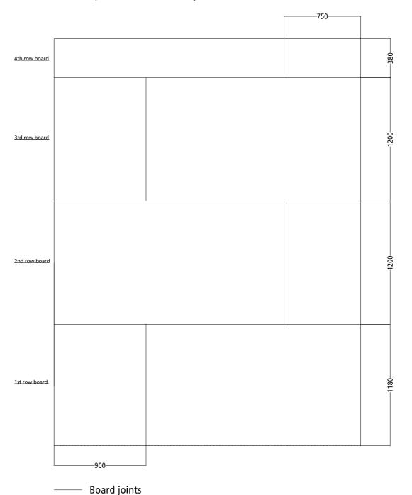
Figure 3 - Exposed face outer layer boards
