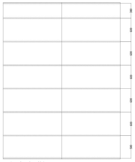
Outer layer board jointsStud positions
