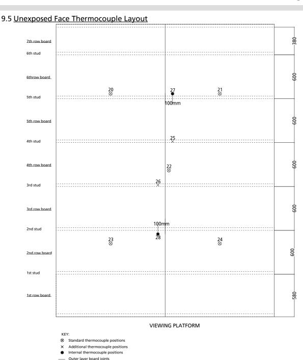
Figure 8 - Unexposed face thermocouple layout
