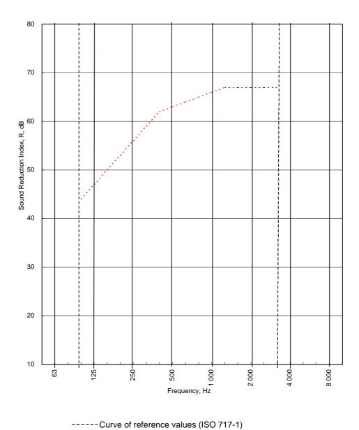
Rating according to RW (C;Ctr) = 63 (-3;-9) dB BS EN ISO 717-1:1997 Max dev. dB at Hz Evaluation based on laboratory  $C_{50-3150}$  = dB  $C_{50-5000}$  = dB  $C_{100-5000}$  = dB measurement results obtained by an engineering method:  $C_{tr,50-3150}$  = dB  $C_{tr,50-5000}$  = dB  $C_{tr,100-5000}$ : dB
