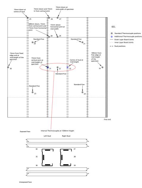
Figure 6. Unexposed face thermocouple layout.
