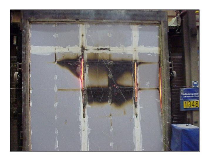
Photograph 5. View of the unexposed face at test termination (119 minutes).
