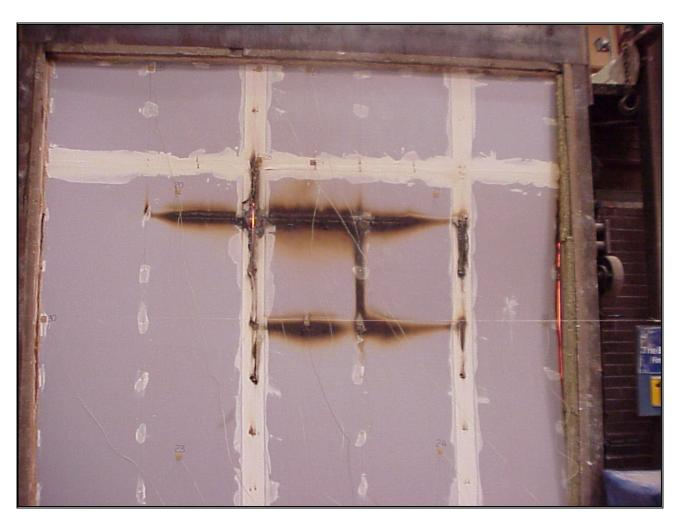
Photograph 4. View of the unexposed face at 114 minutes (after integrity failure).
