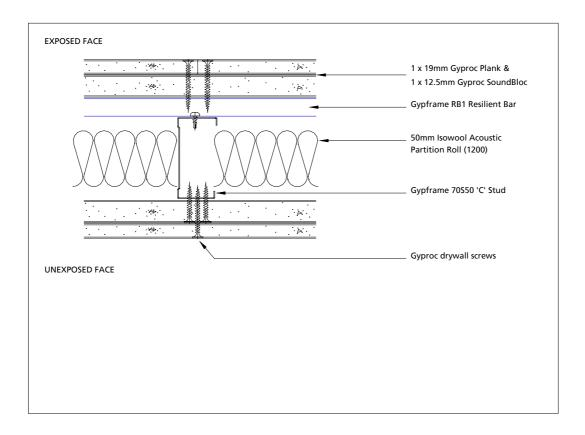
Figure 1. Cross-section of partition specimen.
