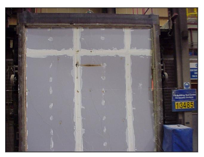
Photograph 3. View of the unexposed face at 106 minutes (after insulation failure).
