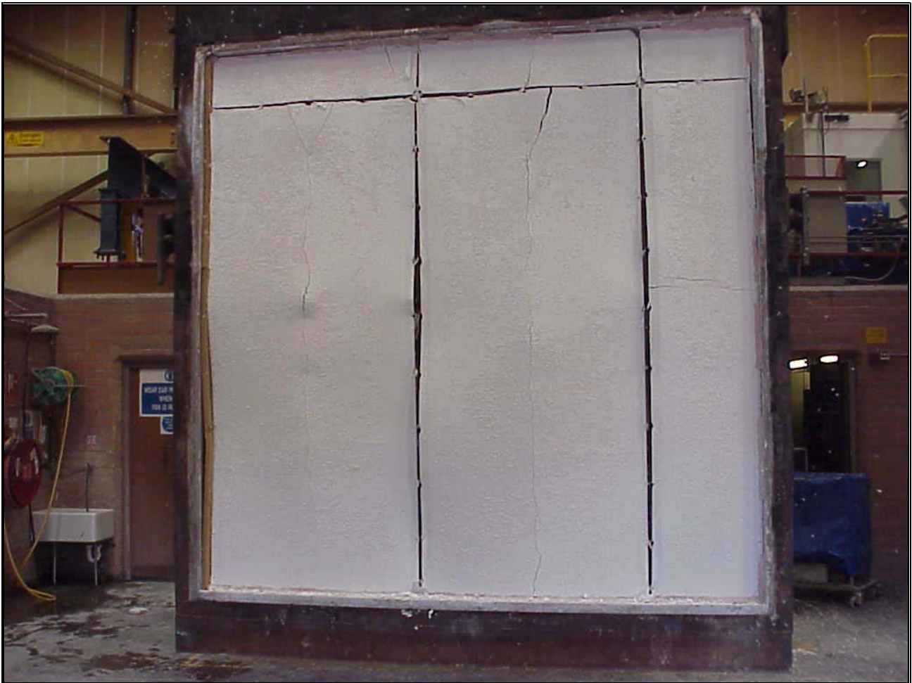
Photograph 4. View of the exposed face after test termination.
