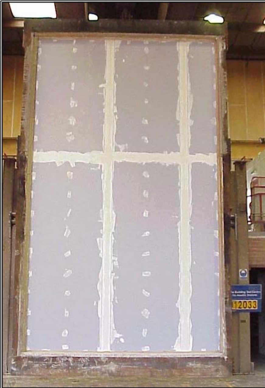
Photo 1. Exposed face prior to test.
