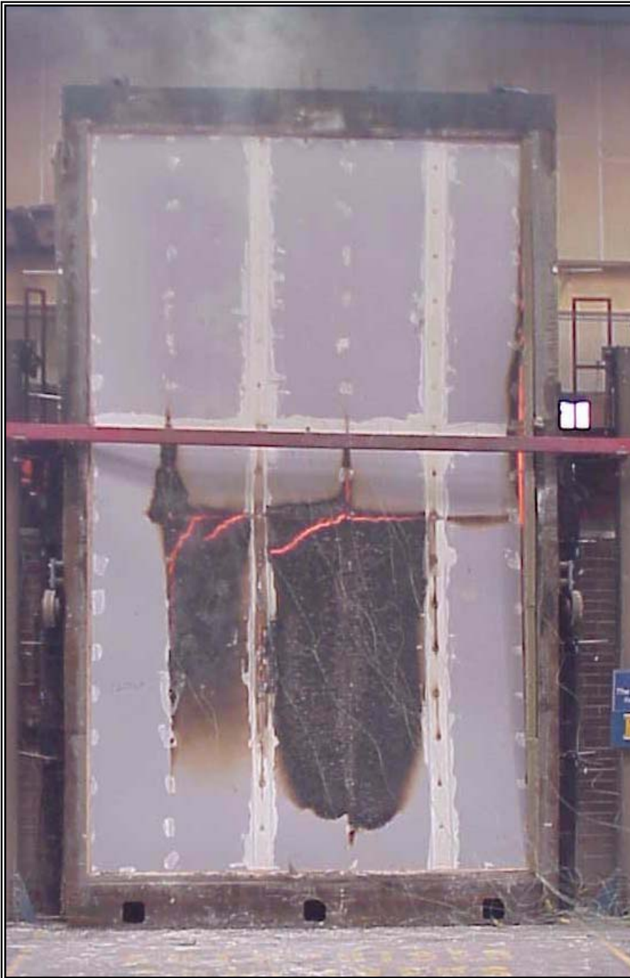
Photo 4. View of the unexposed face at Test Termination.
