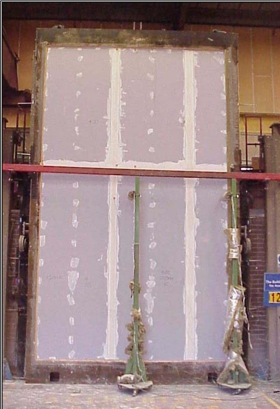
Photo 2. Unexposed face prior to test.
