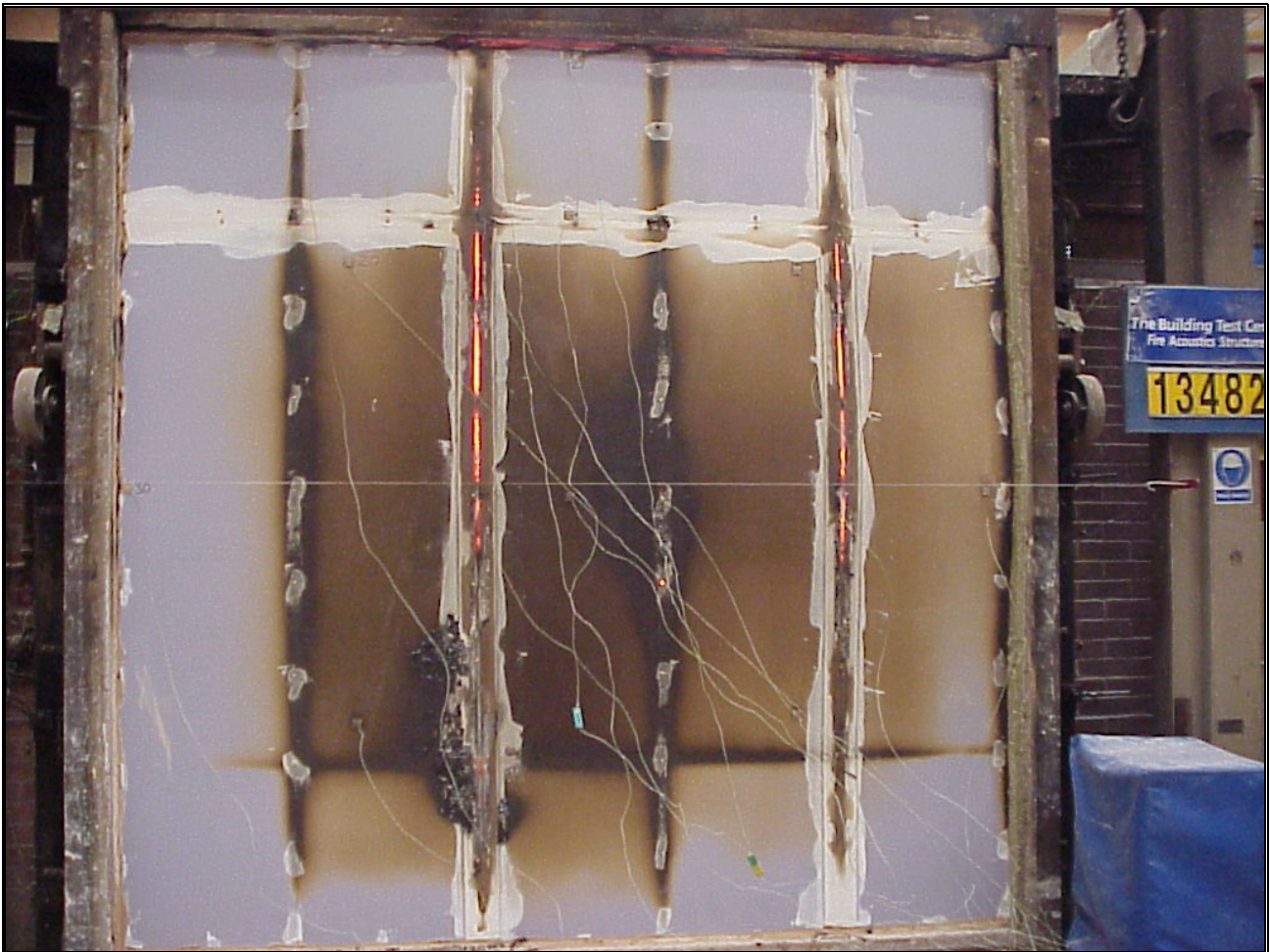
Photograph 5. View of the unexposed face at test termination (125 minutes).
