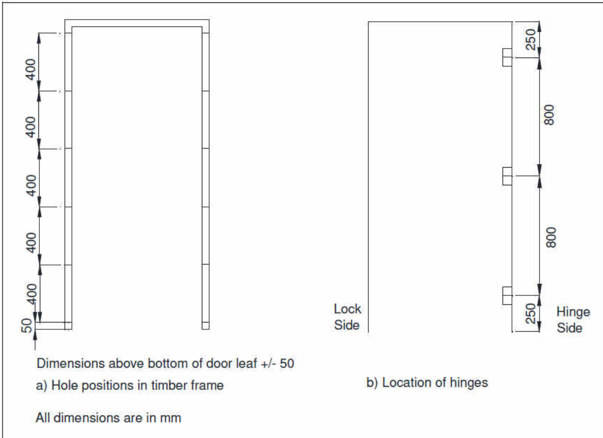
Figure 3. Fixing positions of the door frame.
