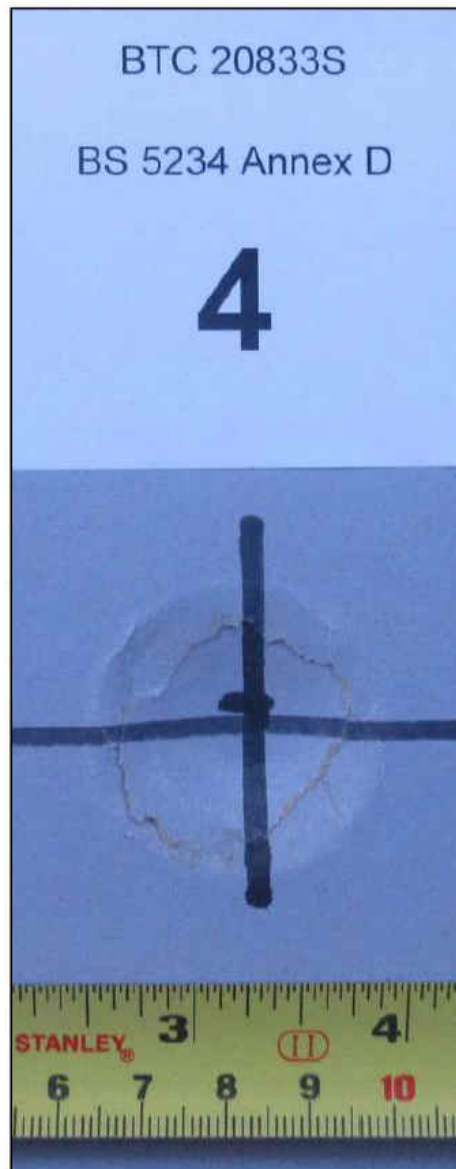
Photograph 1. Example of damage caused by the Annex D – Determination of resistance to perforation by small hard body impact – to partition tested in BTC 20833S
