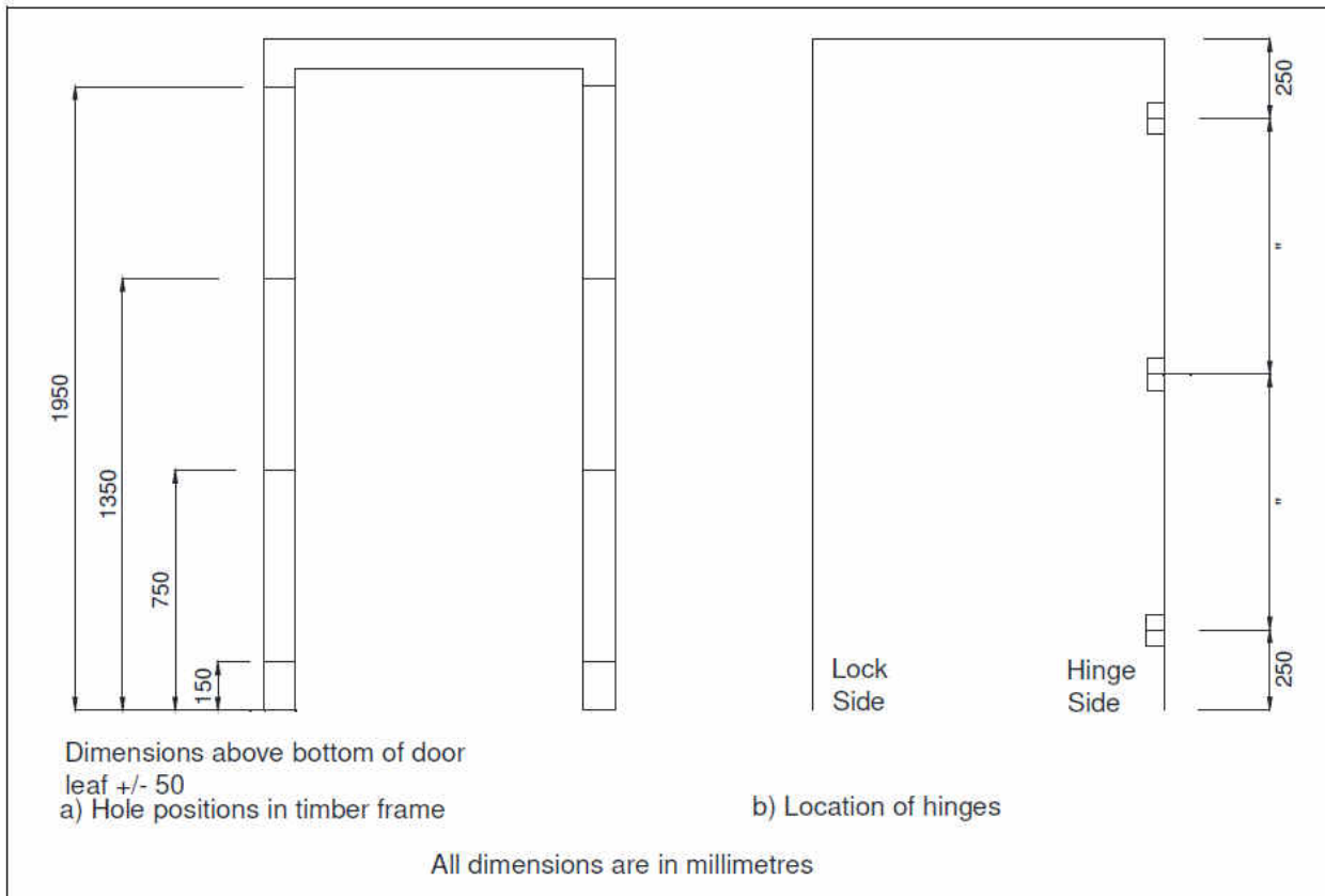
Figure 5. Fixing positions of the door frame
