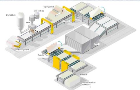
The initial materials are homogenously mixed to form a gypsum slurry that is spread via hose outlets onto a Glass fiber mat on a moving belt conveyor. A second glass fiber mat is fed onto the production line from above to form the plasterboard. The plasterboard continues along the production line where it is finished, dried, and cut to size.
