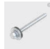
Stainless steel self-drilling insulation fastener screws (4.8mm diameter) Use to attach Polterm Max Plus into the SFS framework. Minimum 10mm threaded penetration into the SFS framework.
