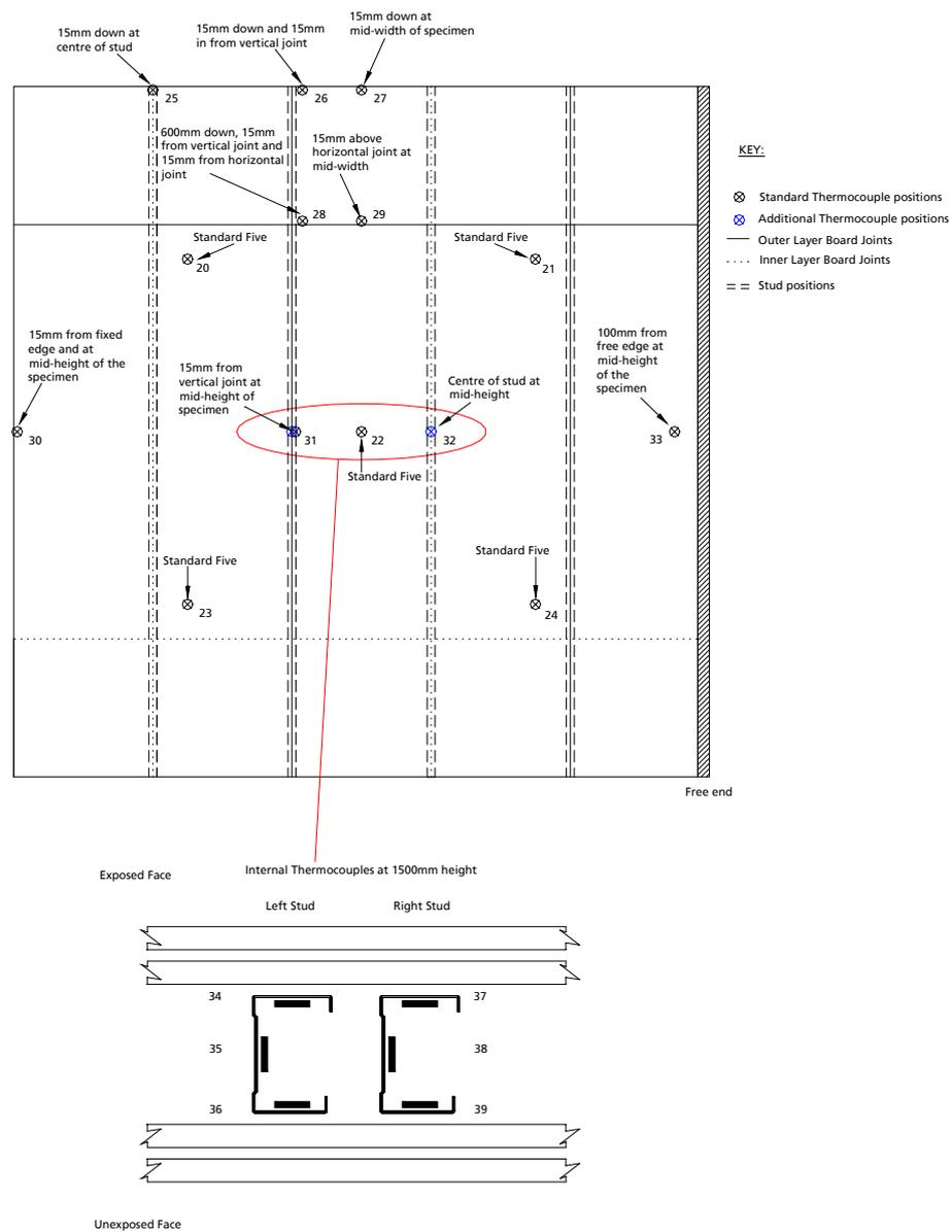
Figure 6. Unexposed face thermocouple layout.
