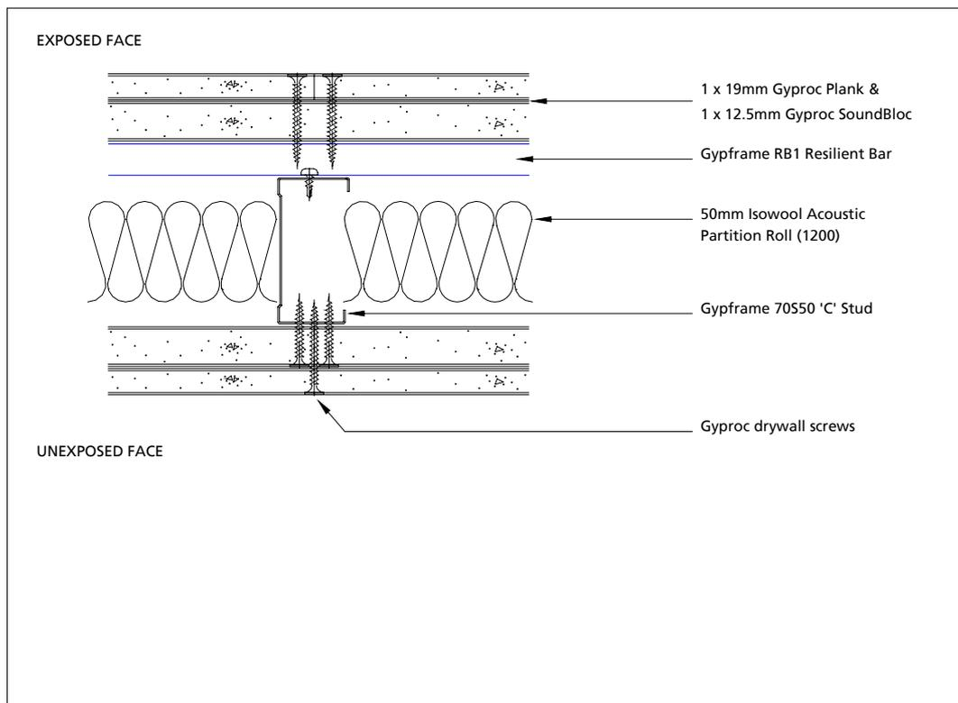
**Figure 1.** Cross-section of partition specimen.
