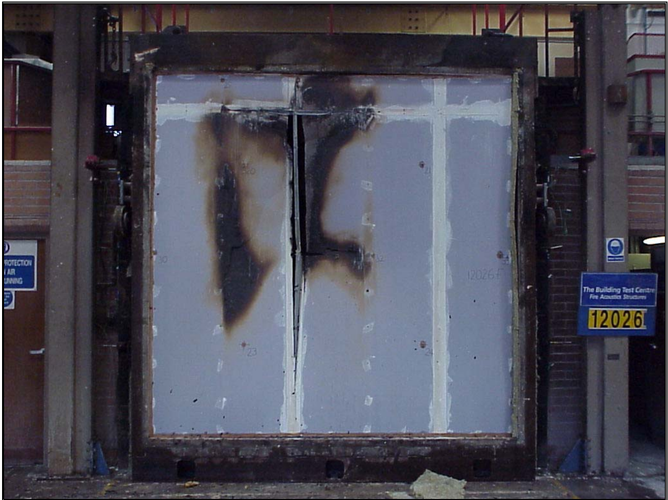
Photo 4. View of the unexposed face after test termination showing areas of insulation and integrity failure.
