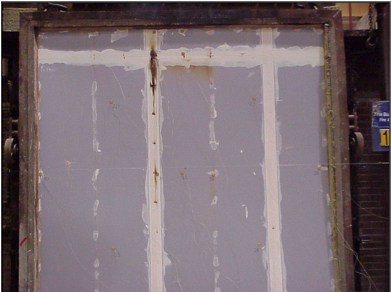
Photograph 3. View of the unexposed face at 58 minutes (after insulation failure).
