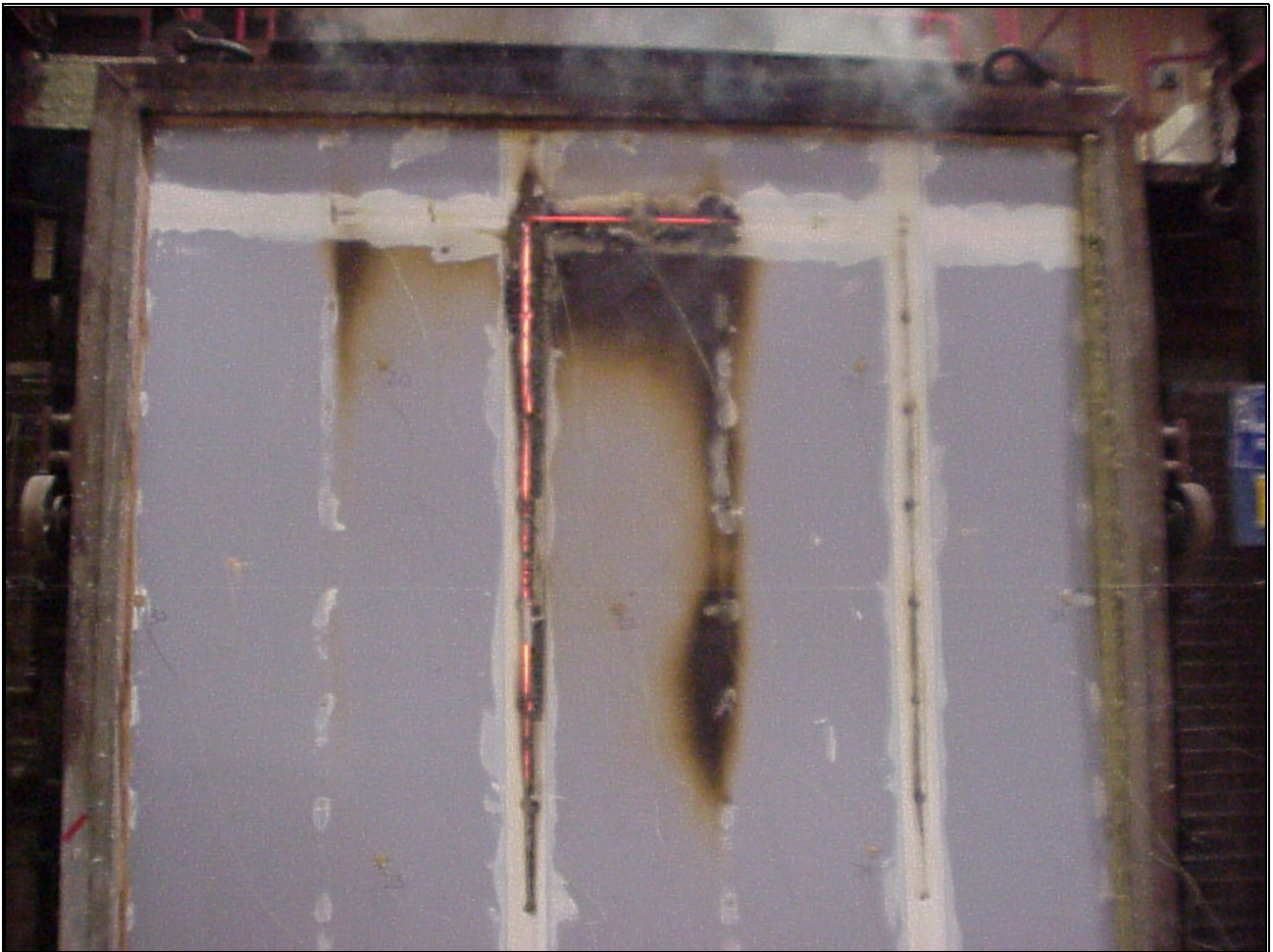
Photograph 4. View of the unexposed face at 64 minutes (after integrity failure).
