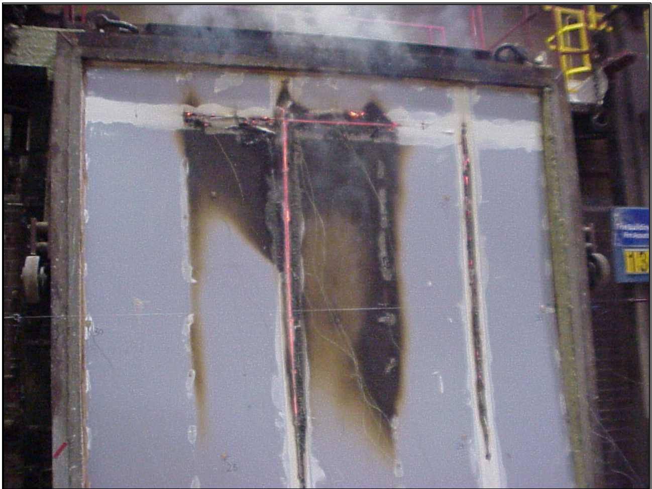
Photograph 5. View of the unexposed face at test termination (66 minutes).
