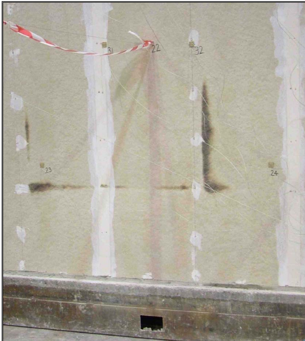
Photograph 3. Position of insulation failure at 82 minutes.
