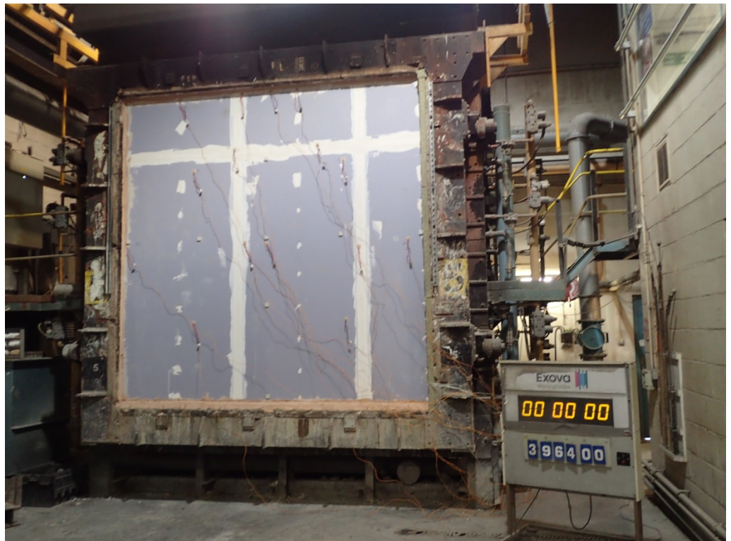
The unexposed face of the specimen prior to the start of the test
