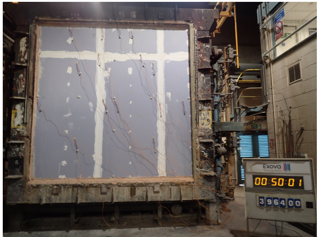
The unexposed face of the specimen after a test duration of 50 minutes
