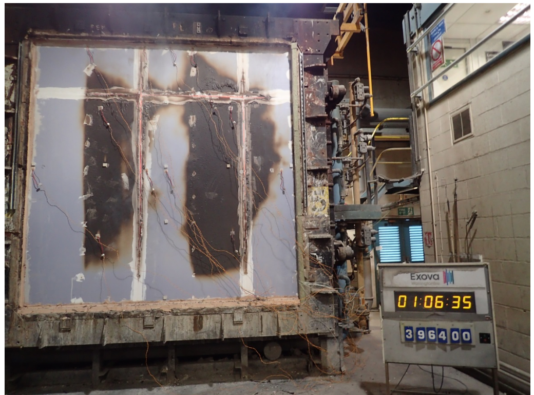
The unexposed face of the specimen after a test duration of 66 minutes
