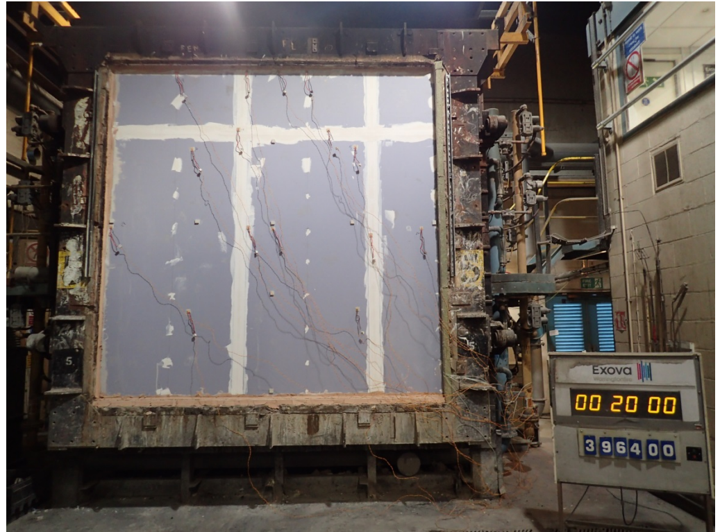
The unexposed face of the specimen after a test duration of 20 minutes
