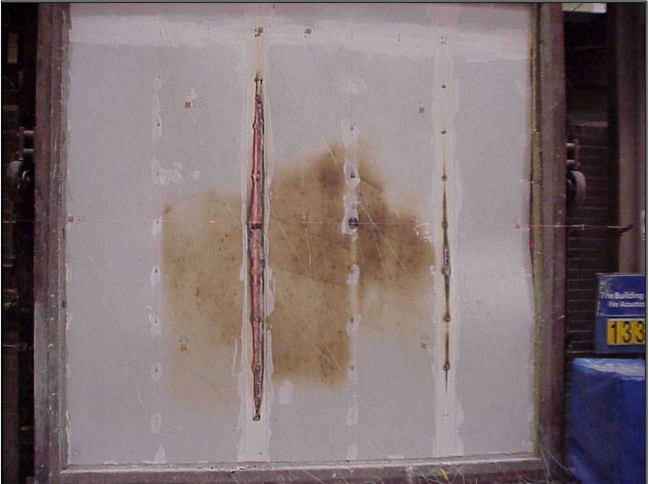
Photograph 3. View of the unexposed face at 42 minutes (after integrity failure).
