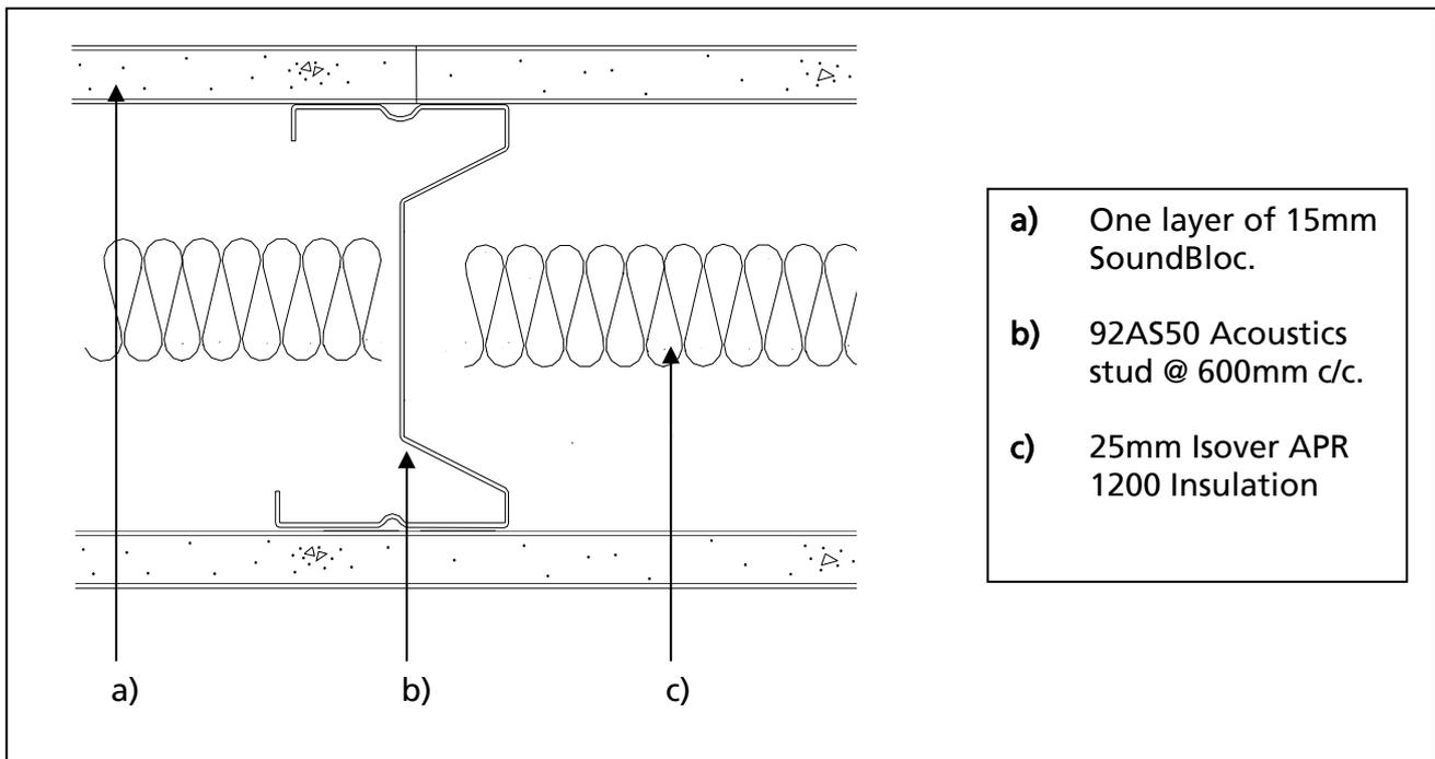
**Figure 1.** Horizontal cross section view through partition BTC16499AA.
