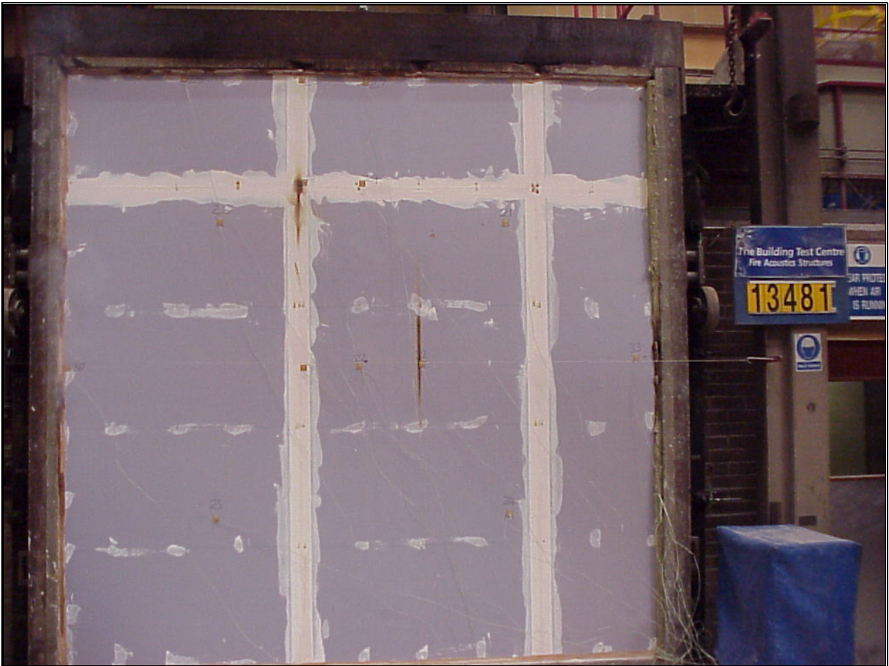
Photograph 3. View of the unexposed face at 101 minutes (after insulation failure).
