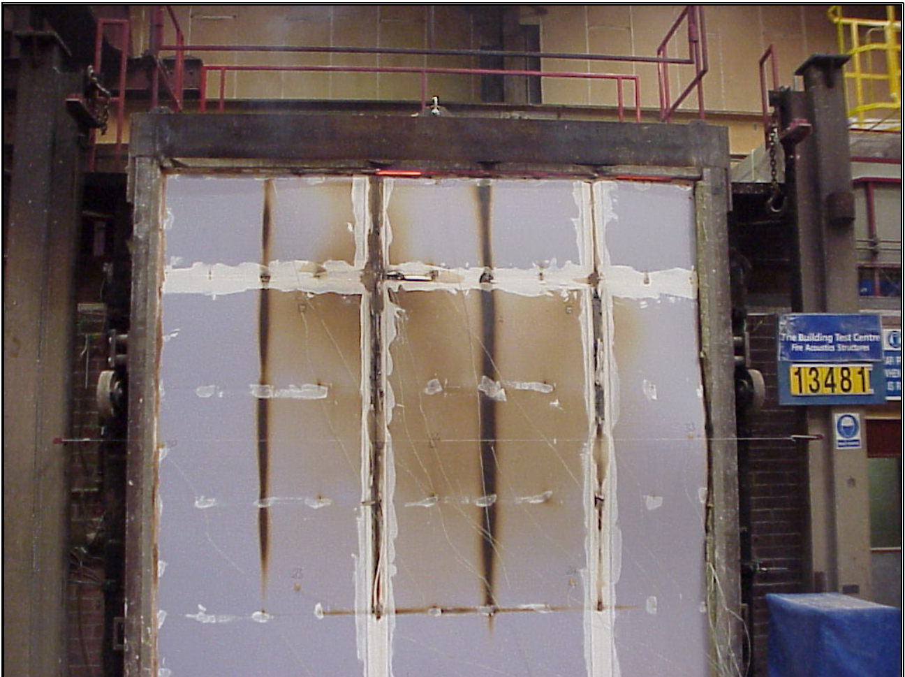
Photograph 4. View of the unexposed face at 117 minutes (after integrity failure).
