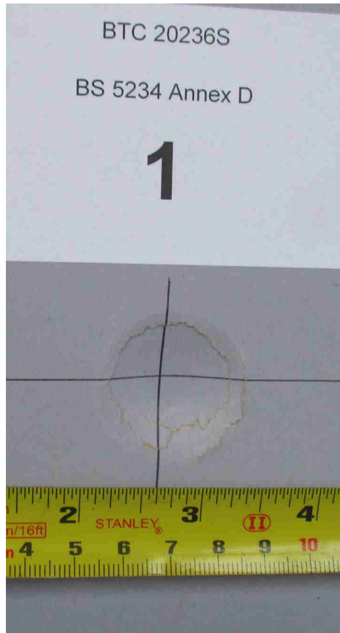
Photograph D.2. Example of damage caused by the Annex D – Determination of resistance to perforation by small hard body impact
