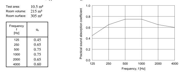
$\label{eq:alpha} \begin{array}{l} \mbox{Practical sound absorption coefficient, weighted sound absorption coefficient, and absorption class according to EN ISO 11654:1997:} \\ \alpha_w = 0.70 \qquad \mbox{Absorption class: C} \end{array}$
