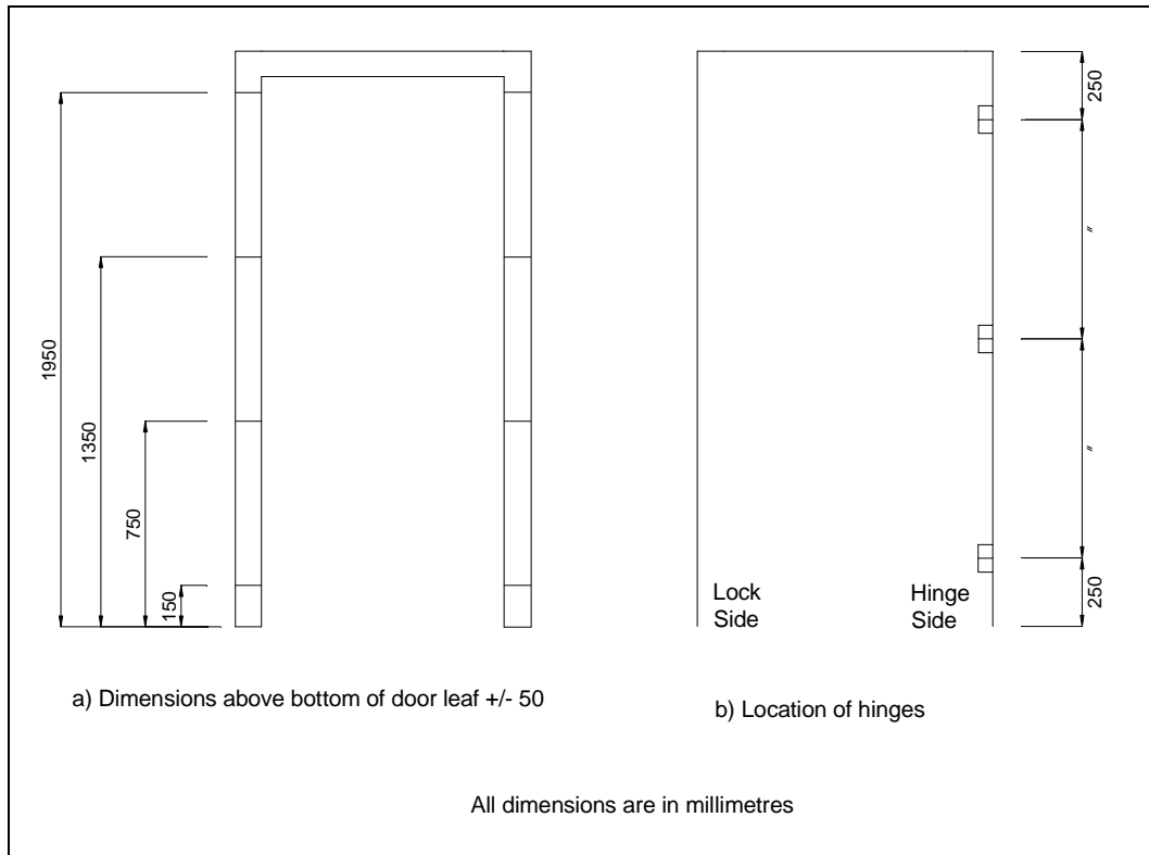
Figure 3 Fixing positions of the door frame
