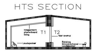
Figure 2. Test Chamber Layout
