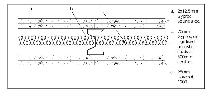
Figure 1. Cross-section through the partition.
