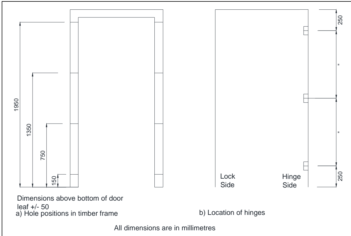
Figure 5. Fixing positions of the door frame
