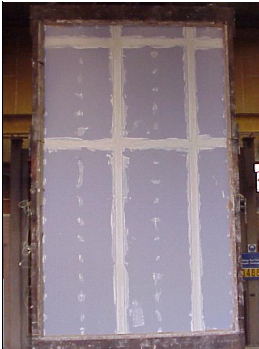
Photograph 1. View of the exposed face prior to test.
