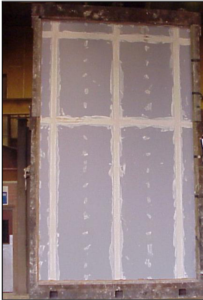
Photograph 2. View of the unexposed face prior to test.
