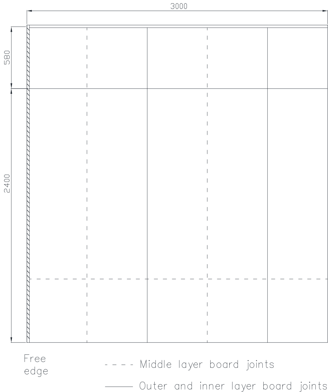
Figure 3 – Unexposed face elevation.
