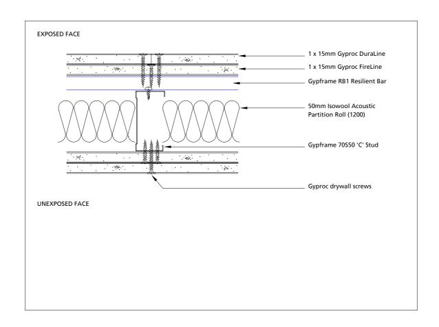
Figure 1. Cross-section through the proposed system (construction 1).
