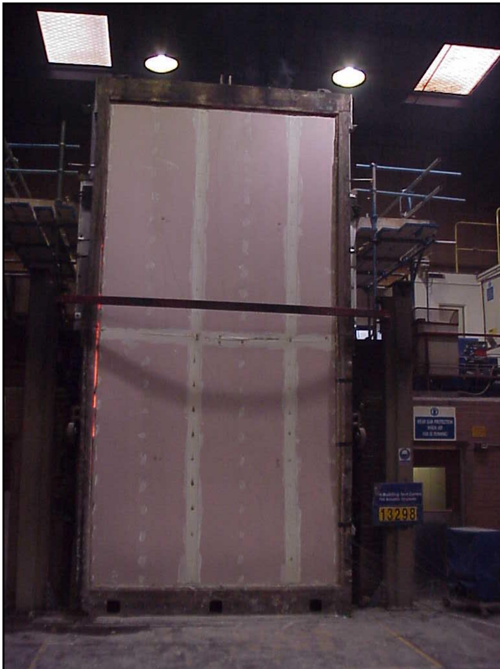
Photograph 2. Unexposed face after 120 minutes duration.
