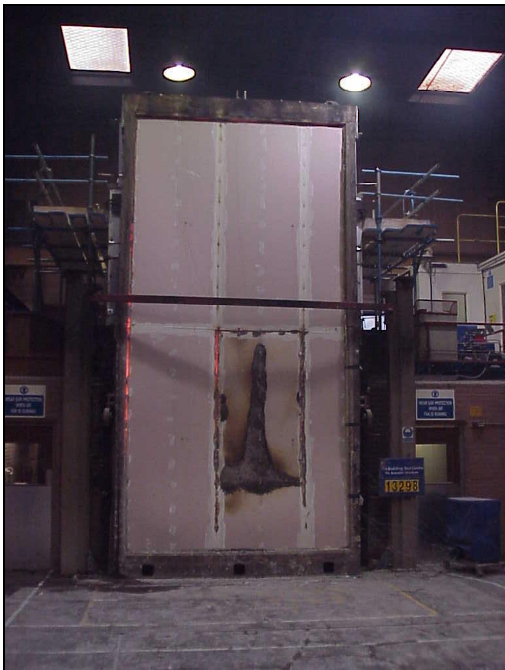
Photograph 4. Unexposed face after test termination at 141 minutes.
