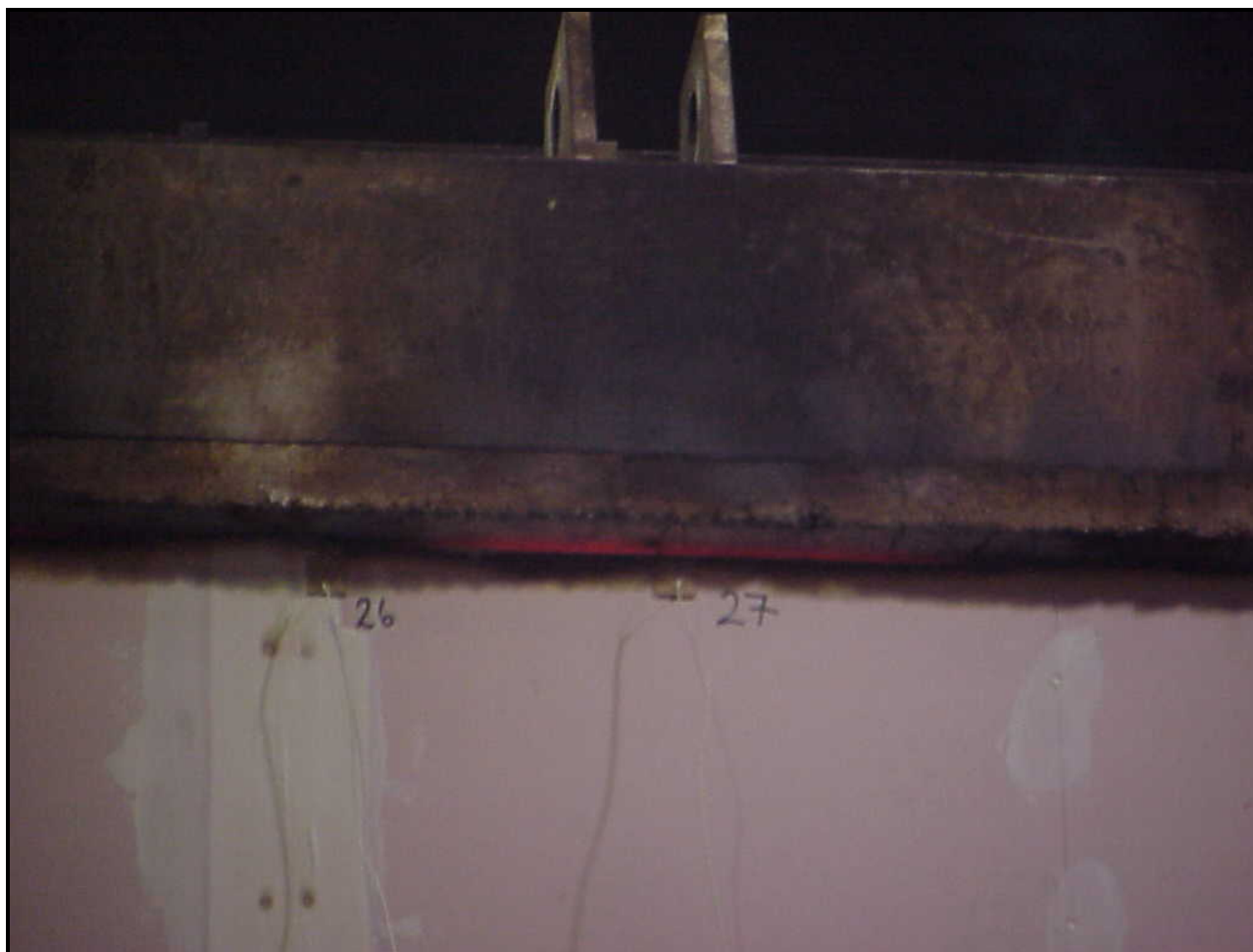
Photograph 3. Position of integrity failure after 123 minutes duration.
