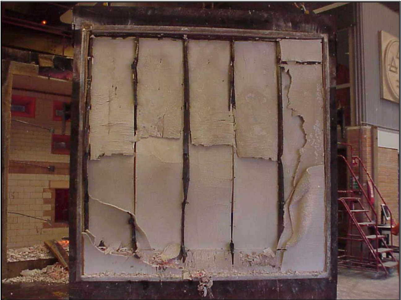
Photograph 4. Exposed face after test termination.
