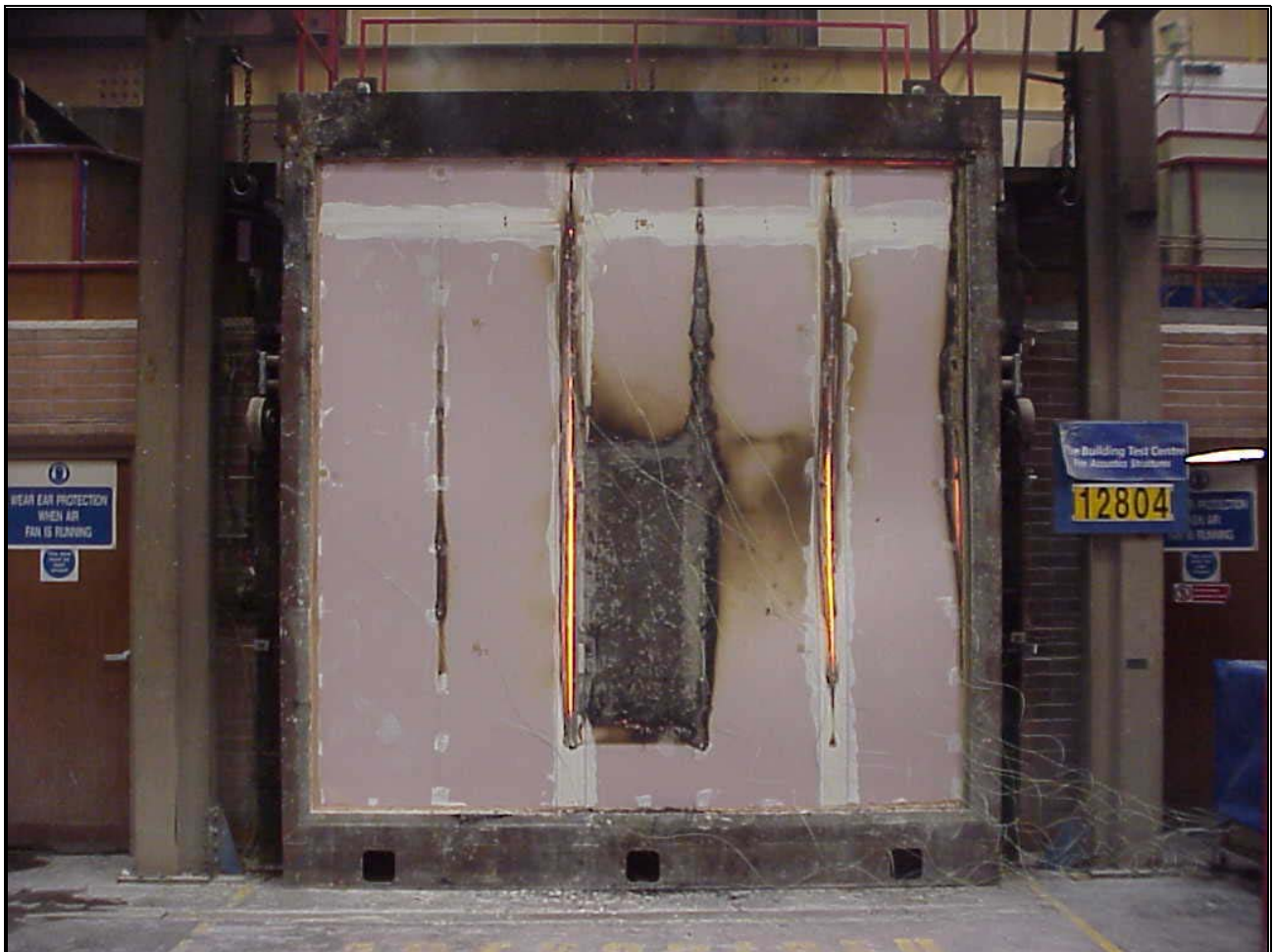
Photograph 3. Unexposed face at test termination.
