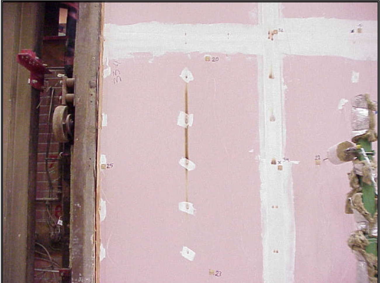
Photo 3. Point of insulation failure in field of board.
