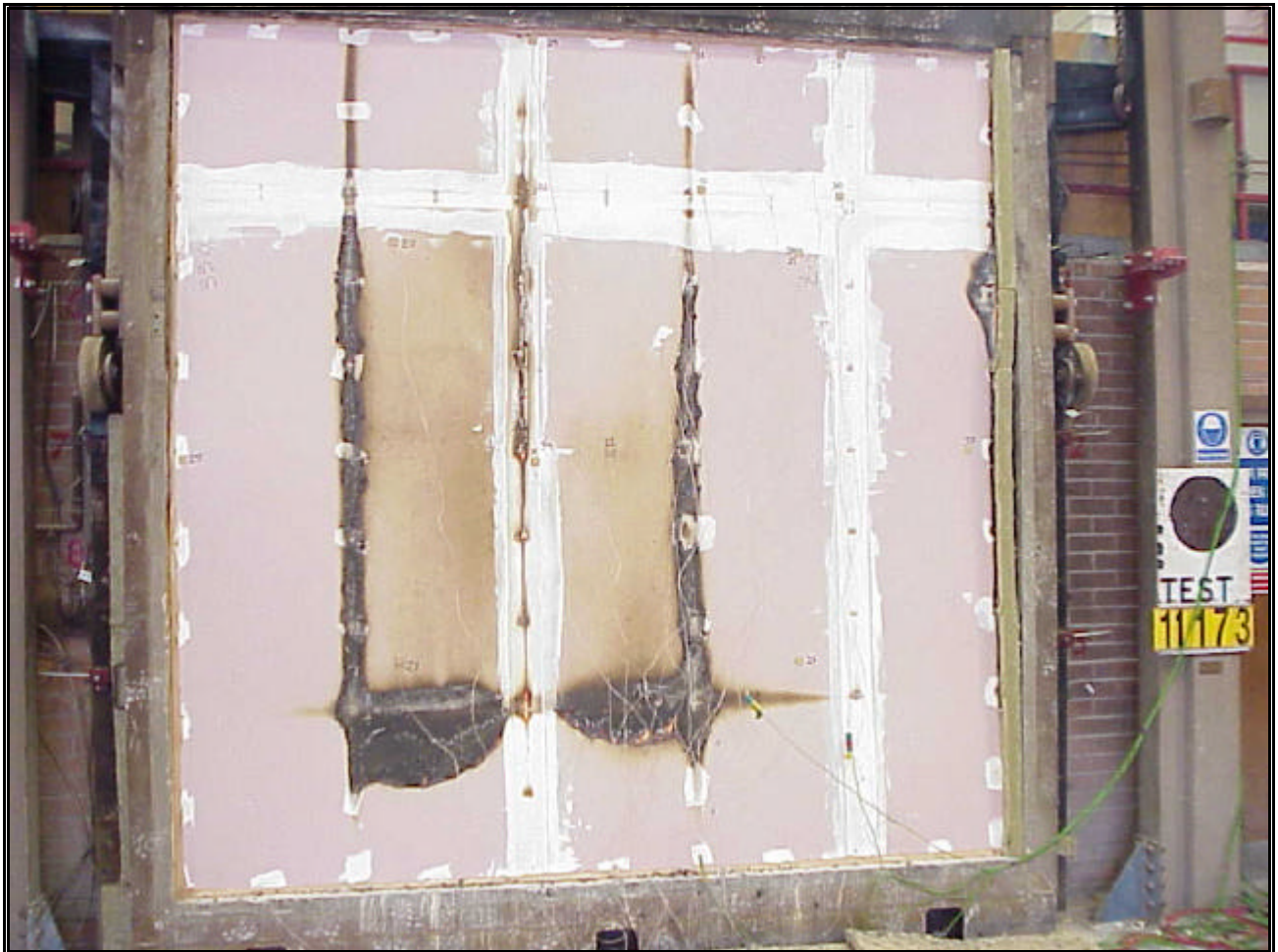
Photo 4. Specimen towards end of test (sustained flaming of paper liner visible)
