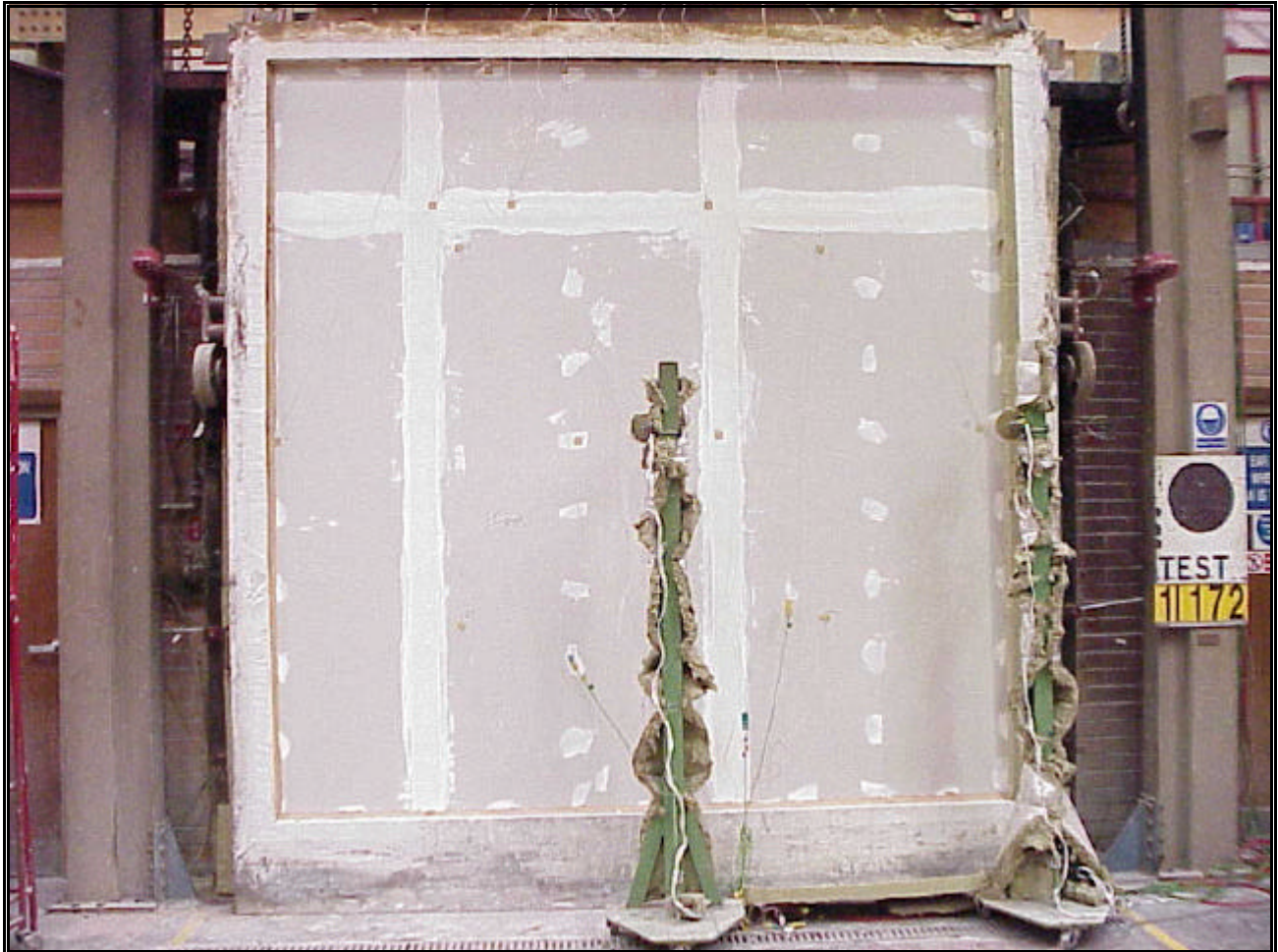
Photo 3. Unexposed face of specimen at 60 minutes.
