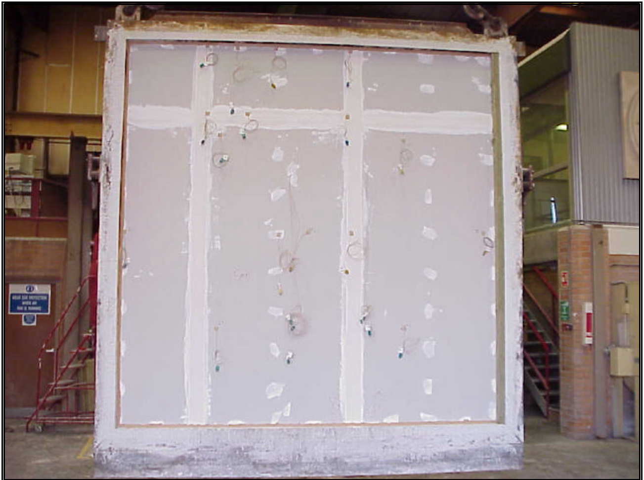
Photo 2. Unexposed face prior to test
