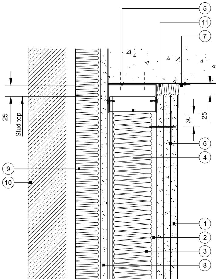
A 25mm designed deflection head gap could accommodate approximately 20mm downward movement. This is due to the stone mineral wool in the head not being able to fully compress
