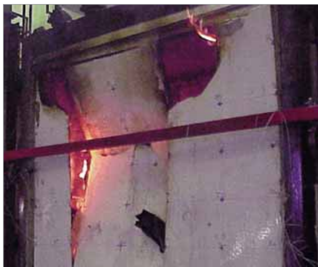
Loaded timber stud wall failing in respect of loadbearing capacity
