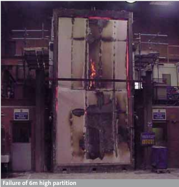
Failure of 6m high partition
